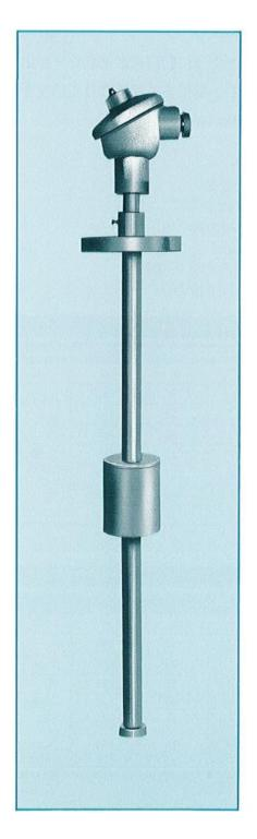
A float with a built-in magnet follows movement of liquid level in tank and turns on/off reed switch inside guide pipe.
